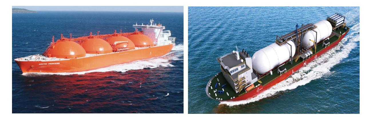
Jamaica imported its first LNG cargoes in 2016 through a new LNG regasification infrastructure delivering to the converted 120 MW Bogue power plant. The process involves a series of ship-to-ship transfers from conventional LNG carriers to a floating storage unit stationed offshore, then to a lightering vessel set to deliver smaller volumes to an onshore regasification receiving centre.
